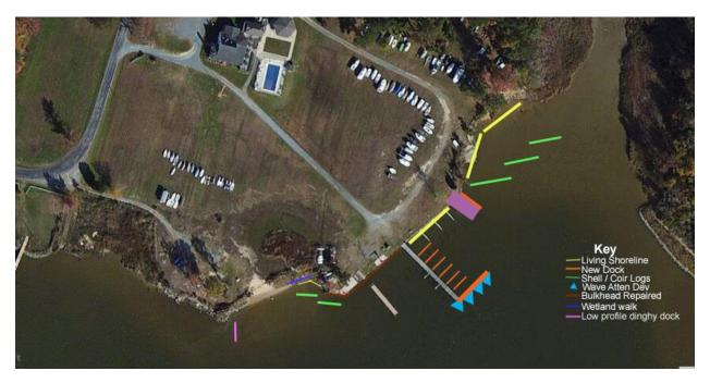
Figure 13. RHYC Waterfront Stabilization Concept
